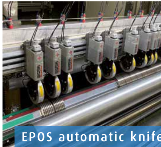
Automatically adjustable upper and lower knives
