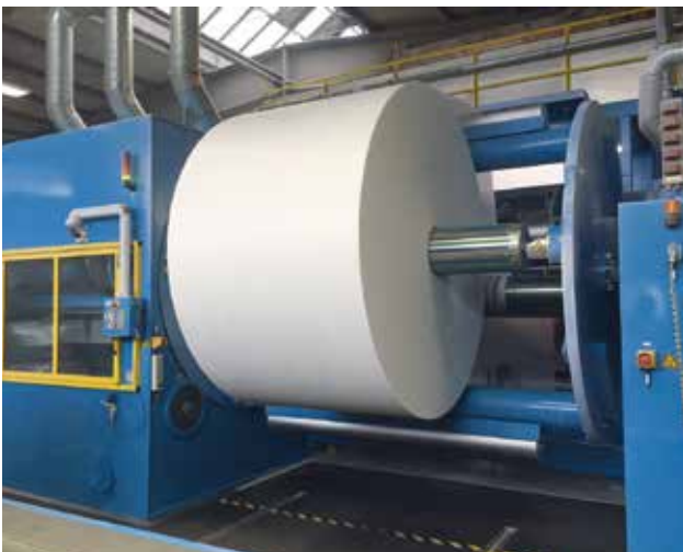
2,400 mm reel in a removal position
