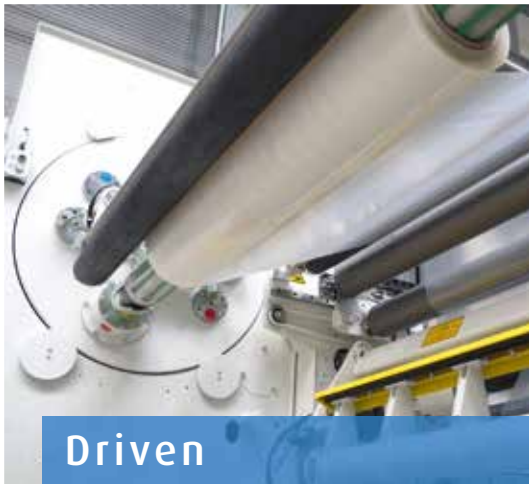
Rider roller on the active winding stations
