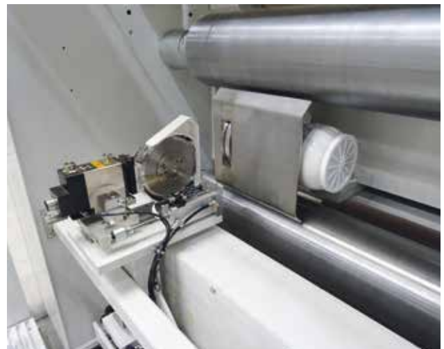
Automatic slitting system with shear cuts and integrated suction
