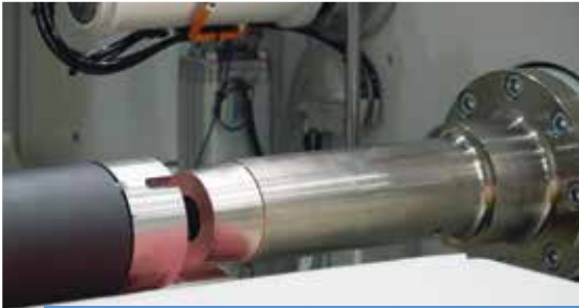
Chuck for a steel winding shaft
