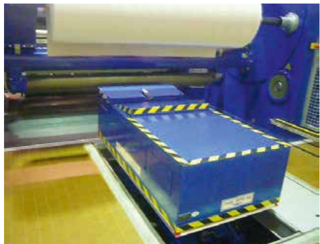
Roll removal with lift table
