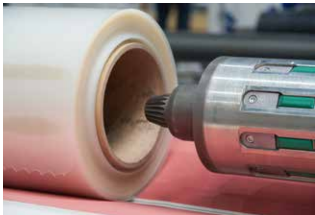
Integrated winding shaft extraction device
