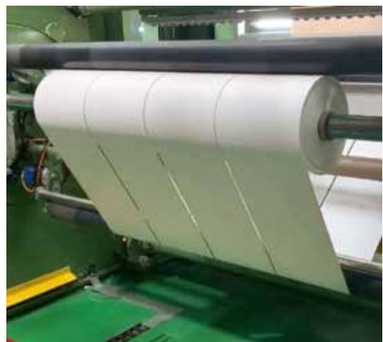
Friction winding for multi-web slitting
