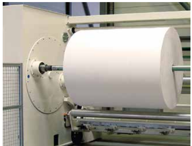
Finished reel in removal position
