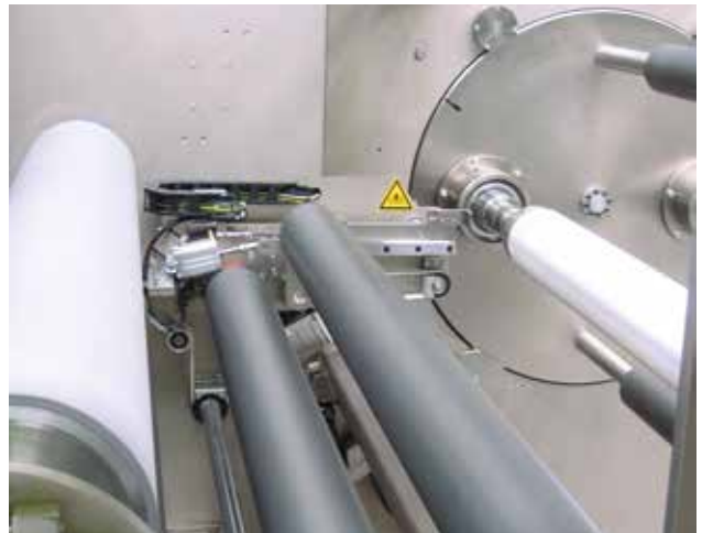
Contact roller carriage
