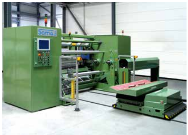
ATW-E with external winding shaft extraction device
