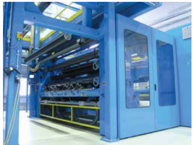
Inlet with integrated pendulum roller and slitting system
