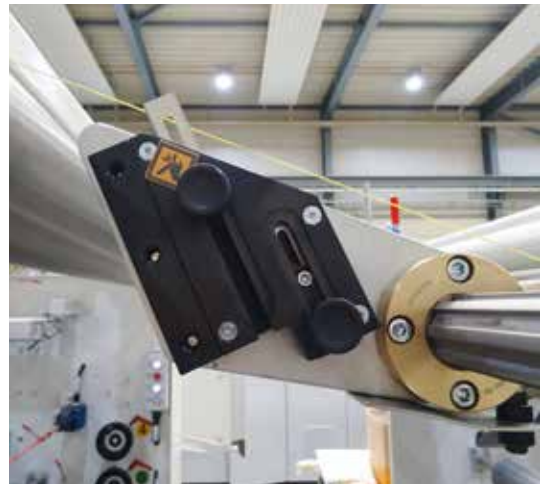
Oscillating blade mounts
