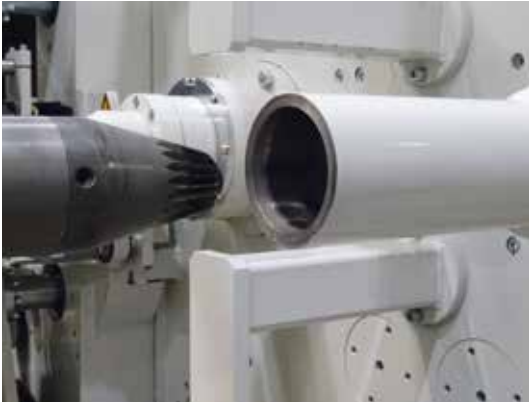
Chuck for a steel winding shaft
