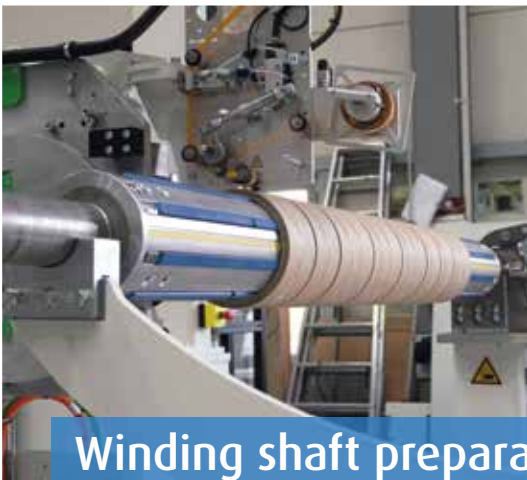
Preparation of winding shaft with automatic application of adhesive
