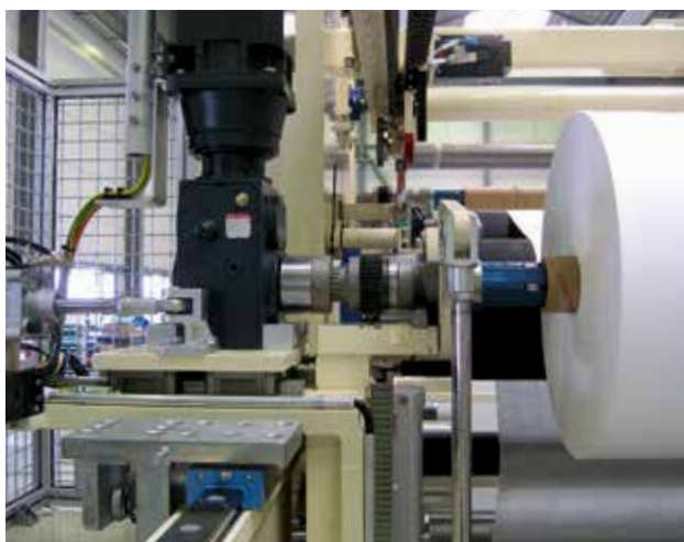
Winding carriage with centre winder
