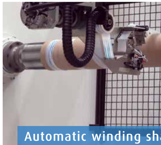
The adhesive tape being applied to the winding shaft
