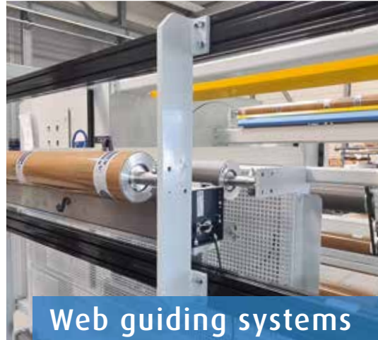
Swivel frame for guiding the web of material
