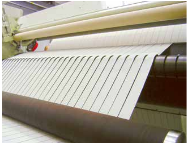
Format roller for consistent gap distances
