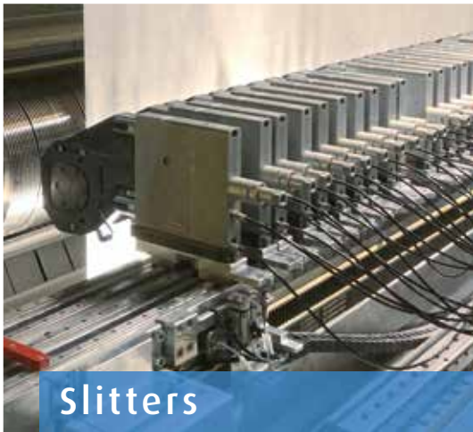
Slitters with the EPOS automatic positioning system
