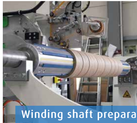
Winding shaft preparation with automatic application of adhesive
